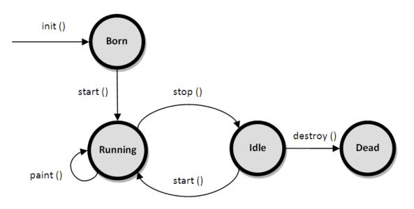
As shown in the above diagram, the life cycle of an applet starts with *init()* method and ends with *destroy()* method. Other life cycle methods are *start()*, *stop()* and *paint()*. The methods to execute only once in the applet life cycle are *init()* and *destroy()*. Other methods execute multiple times.
