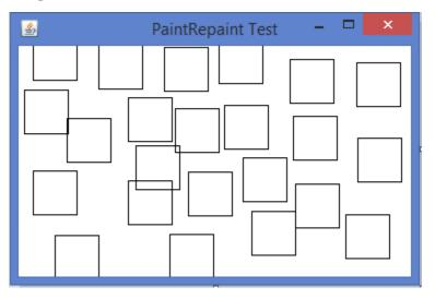
This program involves Frame and event handling mechanism.in which Frame creates a window as shown in output and when you press the mouse the mousepressed event will be occur then it will execute mousePressed method code and run the repaint() method and cursor goes to the paint method and draw a rectangle by using drawRect() method on the window.so we get the multiple rectangles on the window.
